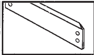
DOUBLE RIVET FRONT TO BACK TIES
